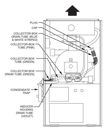
Fig. 6—Alternate Upflow Configuration and Trap Location
